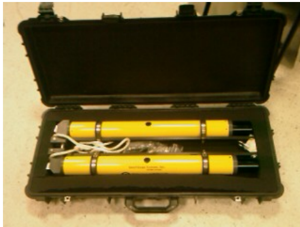
Figure 1.2: Subsurface unit: Model 111 Acoustic Release System (the picture shows 2 releasers in parallel)
