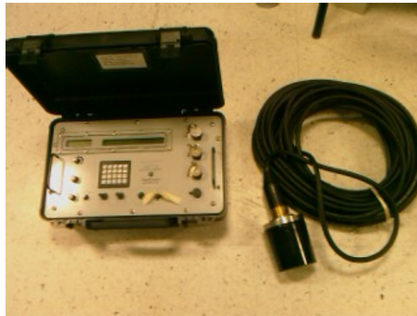
Figure 2.1: Acoustic Command & Ranging Unit Model 1100E and the transponder
