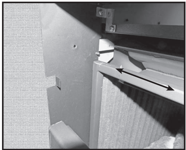
Figure 44: Lip to hang door bracket from.
