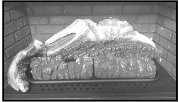
Figure 74: Rustic front logs 3 & 4 installation.
