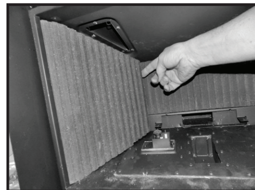
Figure 50: Removing one of the side panels.
