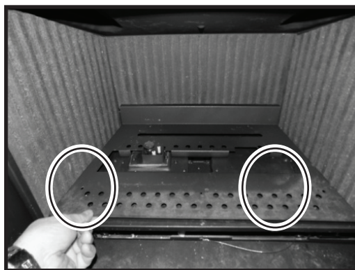
Figure 49: Removing the burner plate.
