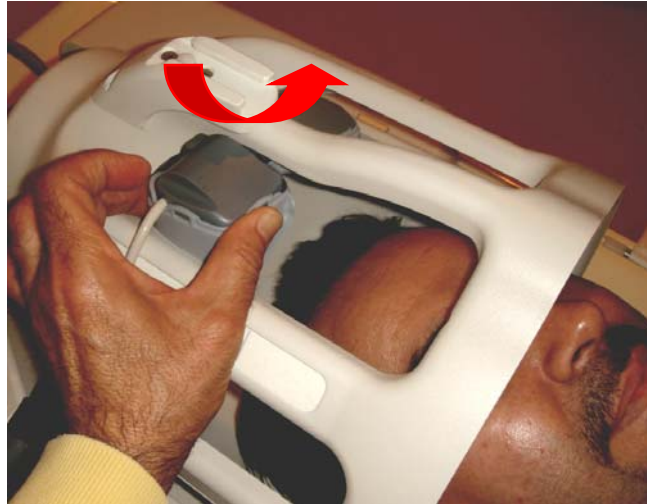
Slide the Video Goggles under the Head coil center part
