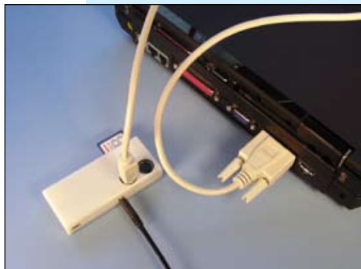
Figure 9-8. Connecting the waysmall computer to a laptop.
