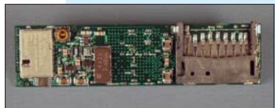
Figure 9-2. Back side of the gumstix board, showing Bluetooth and MMC connectors.
