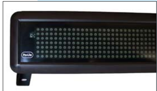
Figure 9-10. Close-up of the Pro-Lite sign showing individual pixels.
