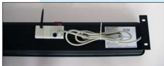
Figure 9-12. Mounting the gumstix to the back of the Pro-Lite sign.
