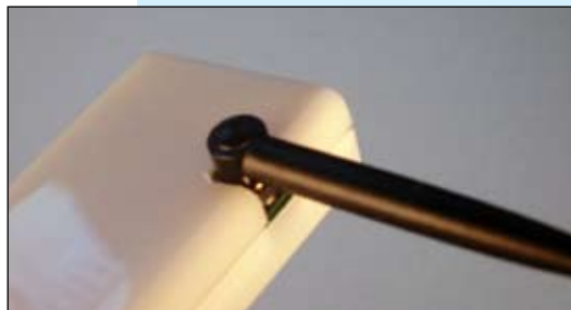
Figure 9-7. The Bluetooth antenna installed.
