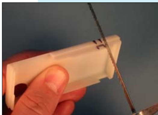
Figure 9-6. Cutting the case with a coping saw.
