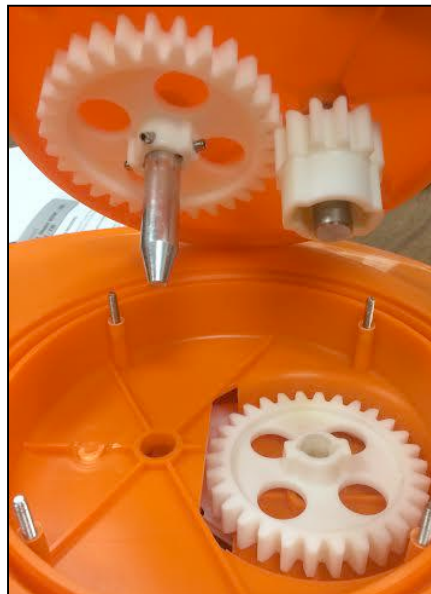
Figure 10 – Salad Spinner with built in gear train.
