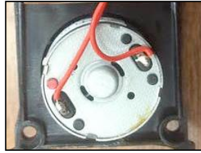
Figure 36 – AC generator in hand crank flashlight
