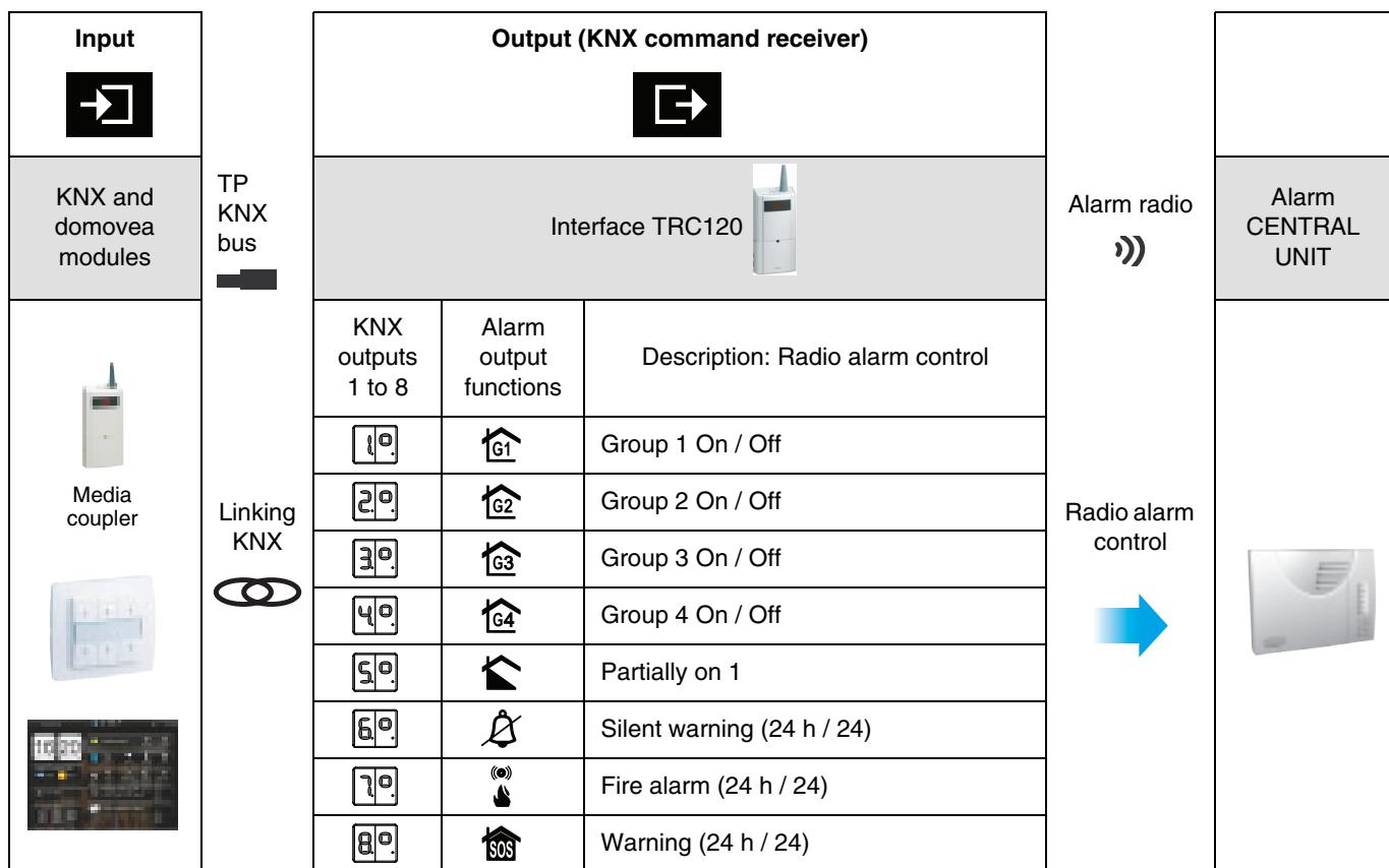
The objects listed above behave like KNX command receivers (Outputs KNX). A **Receiver ON / OFF** and / or **Scene Object** can be associated with each of these 8 controls.
