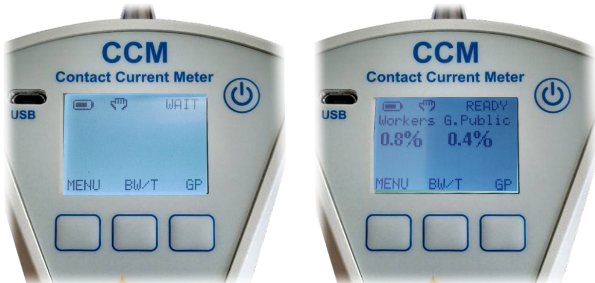
Figure 3.6: Ready for measuring
