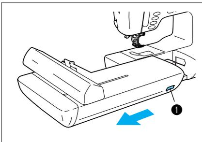
2. Turn off the sewing machine, hold the left side of the embroidery unit, and while pressing the release button, gently slide the embroidery unit away from the machine.
