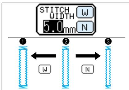
Press the **STITCH ADJUST** key, and then use the **STITCH WIDTH** keys **[W]** and **[N]** to adjust the width of the buttonhole.
