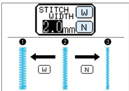
Press the **STITCH ADJUST** key, and then use the **STITCH WIDTH** keys **[W]** and **[N]** to adjust the width of the bar tack.
