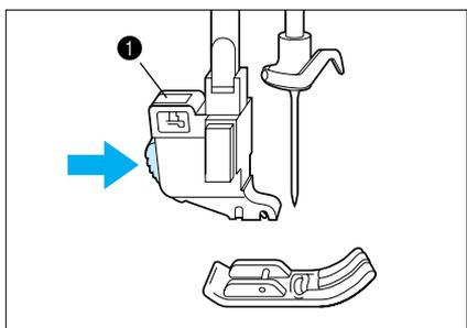
3. Press the black button located at the back of the presser foot holder to release the foot.
