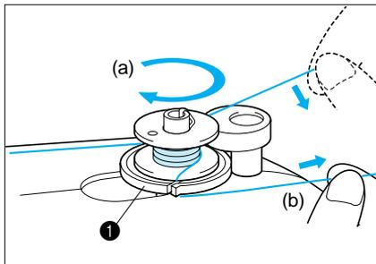
5. Wind the thread clockwise around the bobbin four or five times (a), pass the thread through the slit in the bobbin winder seat, and then pull it as shown to cut it (b).
