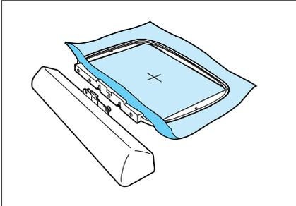
1. Raise the presser foot lever to its highest position, and then pass the embroidery frame under the presser foot, making sure that the mounting bracket of the frame is on the left side and the right side of the fabric is facing up.
