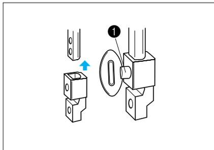
2. Slide the presser foot adapter as high as possible up the presser foot bar, and then fasten it by firmly tightening the screw (for securing adapter) with the enclosed screwdriver or disc-shaped screwdriver.
