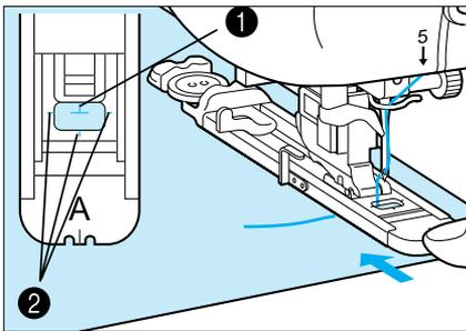
4. Slide the outside frame of the buttonhole foot backward as far as possible as shown in the illustration at the left, making sure that there is no gap behind the part of the foot marked "A".
