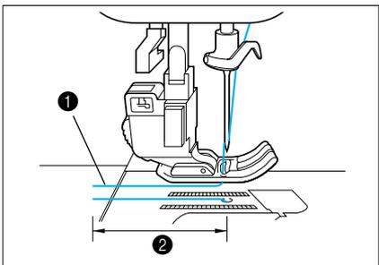
7. Pass the thread underneath the presser foot, and then pull about 2" (5.0 cm) of the upper thread out toward the rear of the machine.
