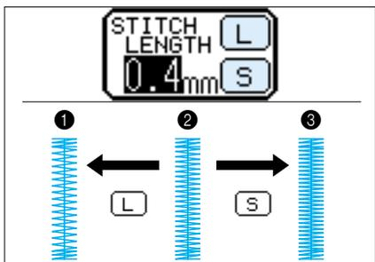
Press the **STITCH ADJUST** key, and then use the **STITCH LENGTH** keys **[L]** and **[S]** to adjust the stitch length of the bar tack.
