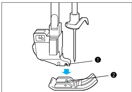
4. Place the other presser foot below the holder so that the presser foot pin is aligned with the slit in the holder.
