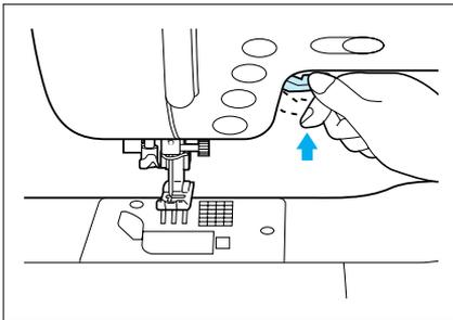
1. Raise the presser foot lever, and then raise it even higher so thicker fabrics can be placed under the presser foot.
