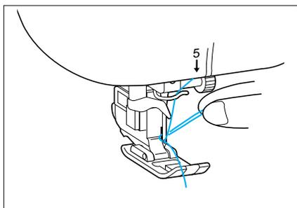
5. Pull the thread through the eye of the needle out towards the rear of the machine.
