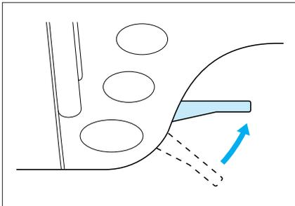
1. Raise the presser foot lever. (If the presser foot is not raised, the sewing machine cannot be threaded correctly.)
