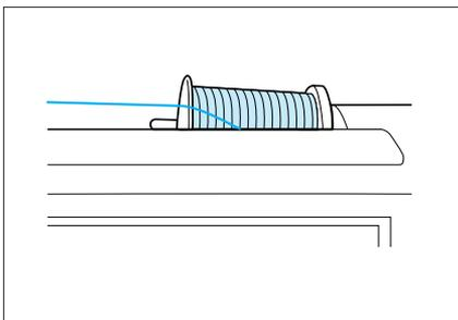
3. Place the spool on the spool pin so that the thread unrolls from the bottom front of the spool. Then, secure the spool on the spool pin using a spool cap with the size closest to the spool size.
