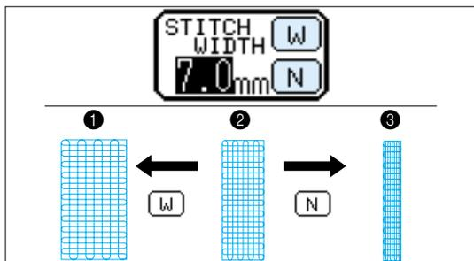
Press the **STITCH ADJUST** key, and then use the **STITCH WIDTH** keys **W** and **N** to adjust the width of the darning.
