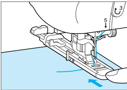
2. Check that the needle drops at the desired position and lower the presser foot lever, making sure that the upper thread passes underneath the buttonhole foot.
