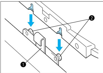
2. Align the slots in the mounting bracket of the frame with the two knobs on the frame holder of the embroidery arm, and then press the frame onto the frame holder so that it clicks into place.
