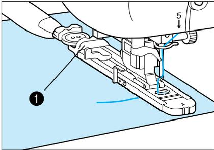
2. Attach buttonhole foot **A** and lower the presser foot lever, making sure that the upper thread passes underneath the buttonhole foot.
