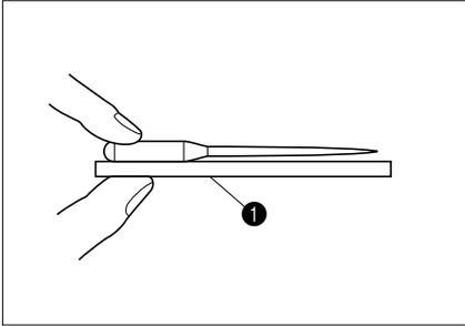
Place the flat side of the needle on a flat surface and check that the needle is not bent up, down, or to either side. If the needle is bent, it should be thrown away to prevent damage to your project or to the machine.
