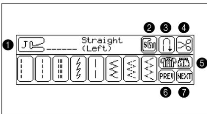
1. When the sewing machine is turned on, the straight stitch (left needle position) is automatically selected.
