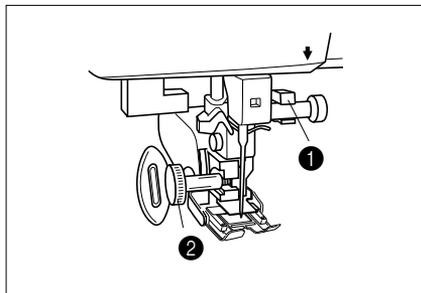
3. Hook the connecting fork of the walking foot onto the needle clamp screw, lower the presser foot lever, and then fasten the walking foot by firmly tightening the screw (for securing presser foot) with the enclosed screwdriver or disc-shaped screwdriver.
