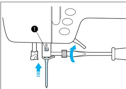
5. With the flat side of the needle facing toward the back, insert the needle as far up as possible so that it touches the needle stopper. Fasten the screw securely with a screwdriver.
