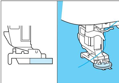
2. Attach button sewing foot **M**, place the button into the presser foot, and then lower the presser foot lever.
