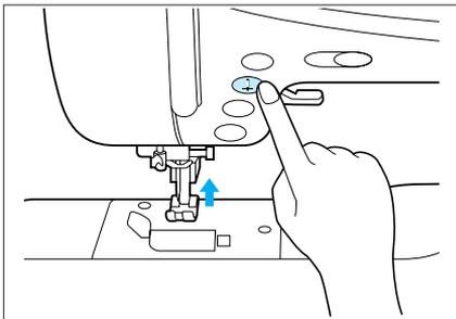
2. Press the needle position button to raise the needle.
