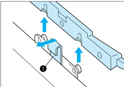
While pushing the release lever on the frame holder to the left, lift the embroidery frame up to remove it.
