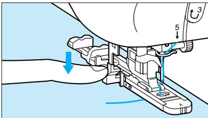
4. Lower the buttonhole lever so that it is positioned behind the metal bracket on the buttonhole foot.
