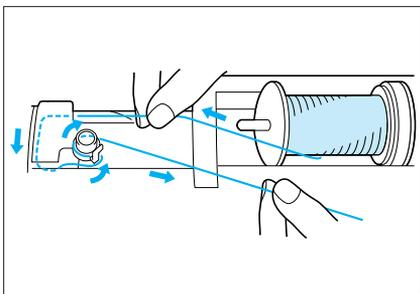
3. While holding the spool thread with your right hand, use your left hand to pass the thread through the guides as shown.
