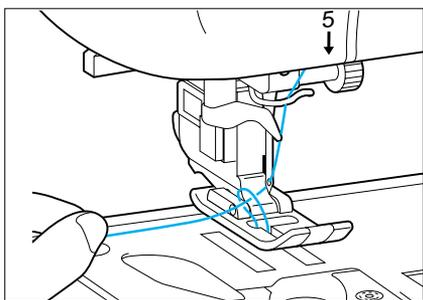
4. With the bobbin cover still removed, hold the upper thread, press the needle position button twice, and then pull up the bobbin thread.
