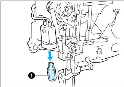
4. Replace the snap-in light bulb with a new one.
