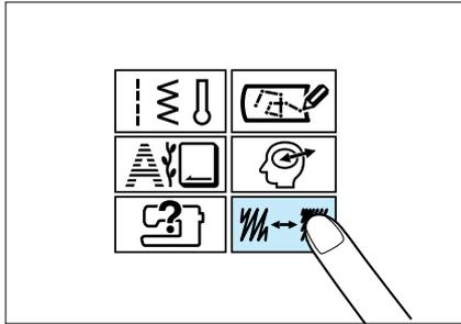
1. Press the **STITCH ADJUST** key, and then select the eyelet size.
