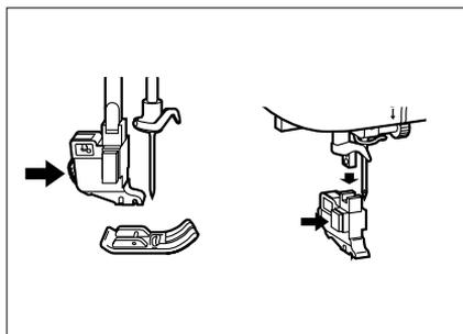
1. Remove the installed presser foot and the presser foot holder.
