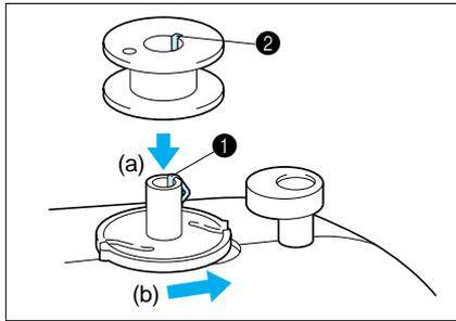
4. Place the bobbin on the bobbin winder shaft so that the spring on the shaft fits into the groove in the top of the bobbin (a). Then, slide the bobbin winder shaft to the right (b).
