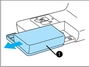
With the flat-bed attachment removed, sewing tubular pieces, such as sleeves and pant legs, or hard-to-reach areas of the garment is easier. To remove the flat-bed attachment, pull it straight out to the left of the sewing machine.
