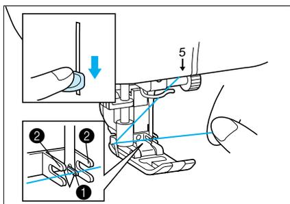
2. Lower the needle threader lever to its lowest position and check that the thread is held by the large hook and that the small hook has passed through the eye of the needle.
