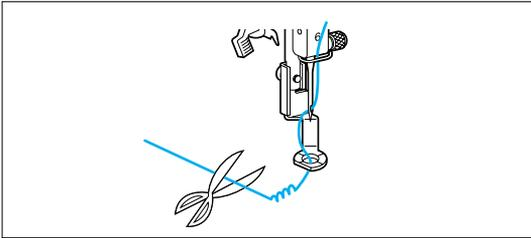
1. After threading the bobbin thread, the upper thread and the needle, pass the thread down through the hole in embroidery foot **Q**, and then pull about 2" (5 cm) of the upper thread out toward the rear of the machine.
