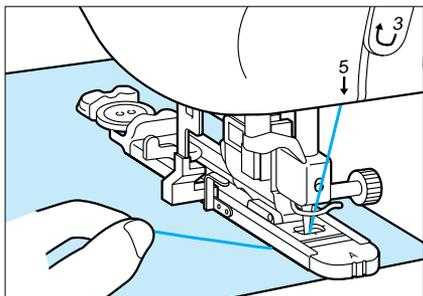
7. Gently hold the end of the upper thread, and then start sewing. Feed the fabric carefully by hand while the buttonhole is sewn. Once sewing is completed, the machine automatically sews reinforcement stitches, and then stops.
