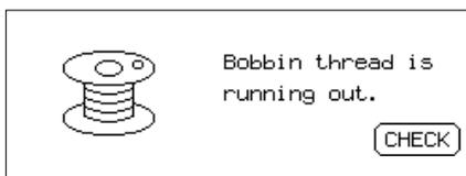
This message appears when the machine detects that the amount of bobbin thread remaining is low.
