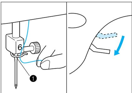
5. Pass the thread through the wire loop, and then lower the presser foot lever.
