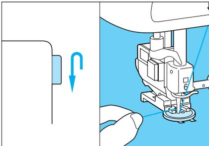
4. Gently hold the end of the upper thread, turn the balance wheel to check that the needle correctly goes into each hole in the button, and then start sewing. Once sewing is completed, the machine automatically stops.
