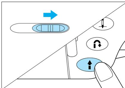
6. Slide the sewing speed controller to its maximum (as far as possible to the right).
