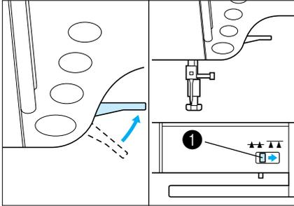
1. Raise the presser foot lever and slide the feed dog position switch to the right to lower the feed dogs.
