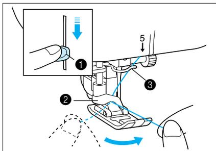
1. Use your left index finger to lower the needle threader lever while gently pulling the thread to the left so that it catches on the large hook.
