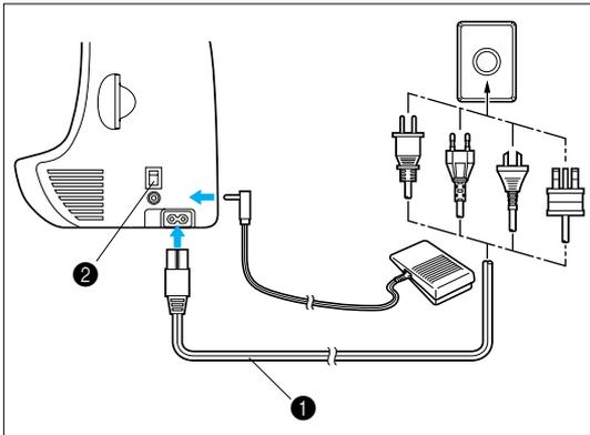
1. Pull out the power supply cord and insert the plug into a wall outlet.
