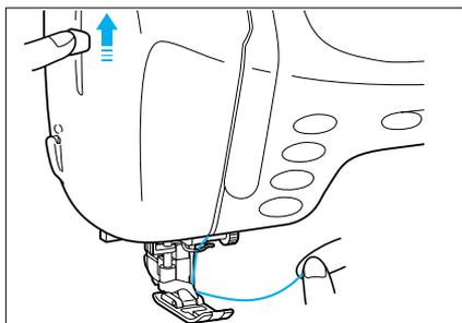
4. While gently holding the thread, raise the needle threader lever.
