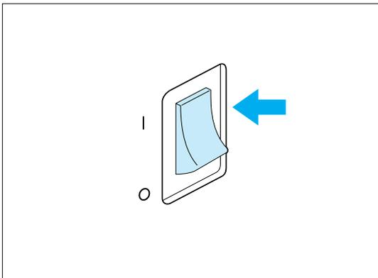
2. To turn on the machine, set the main power switch to "I".
