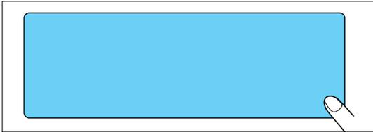
1. While pressing anywhere in the LCD, turn the sewing machine off, then back on again.
