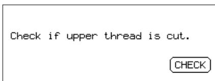
This message appears when the machine detects that either there is no upper thread or it is cut. If the upper thread is cut, re-thread it.
