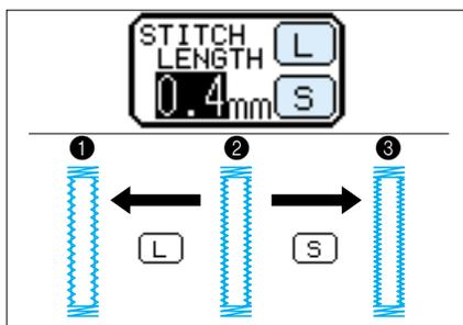
Press the **STITCH ADJUST** key, and then use the **STITCH LENGTH** keys **[L]** and **[S]** to adjust the stitch length of the bar tacks.
