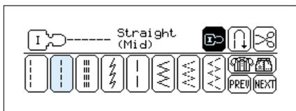
3. Press [Straight (Mid)], and then press (presser foot **I**). The thread tension automatically adjusts for presser foot **I**.
