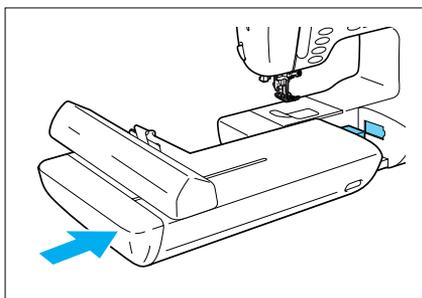
3. Insert the connector on the embroidery unit firmly into the connecting slot.
