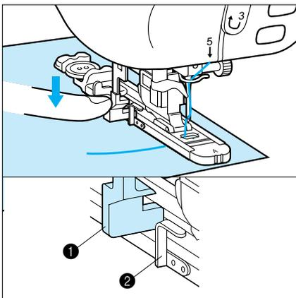
6. Lower the buttonhole lever so that it is positioned behind the metal bracket on the buttonhole foot.
