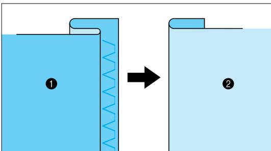
Press the **STITCH ADJUST** key, and then use the **STITCH WIDTH** keys **W** and **N** to adjust the needle position so that the needle slightly catches the fold of the hem.
