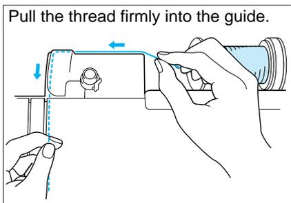
4. While holding the spool thread with your right hand, use your left hand to keep the thread taut while passing it through the guides as shown.
