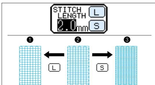
Press the **STITCH ADJUST** key, and then use the **STITCH LENGTH** keys **L** and **S** to adjust the stitch length of the darning.
