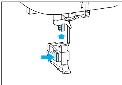
4. While pressing the black button on the left side of the presser foot holder, slide the holder as high as possible up the presser foot bar, and then release the button.
