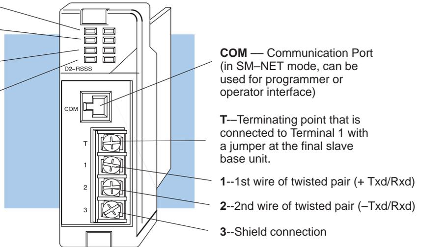
**COM** — Communication Port (in SM-NET mode, can be used for programmer or operator interface)
