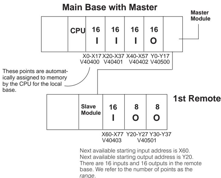
The following is the section of the setup logic which sets up the total input and output ranges for the channel
