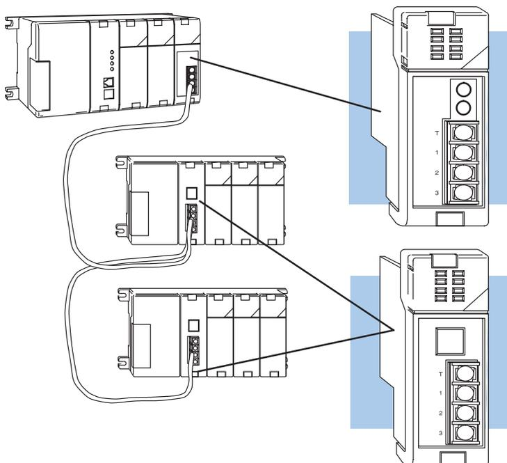
**Remote Master** – The D2-RMSM is mounted in the CPU base. Up to two master modules can be used with the DL240; up to seven master modules can be used with the DL250
