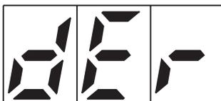
The disk is damaged and it will not be possible to carry out the operation. Press [ESC] to return to the Main Page.
