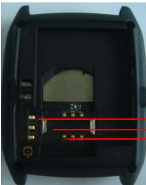
Line up the 3 connectors on battery with these 3 connections.
