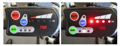
The "On/Off" button turns on/off the control module, the "Mode" button is used to vary the level of assistance and the "Light" button is used to turn the lights on/off.
