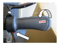
On the left side of the handlebars is the control module. This is used to turn the motor on/off and also to increase/ decrease the amount of assistance given from the electric motor. This module also indicates the **voltage** status of the battery and is used to switch the bike lights on/off.
