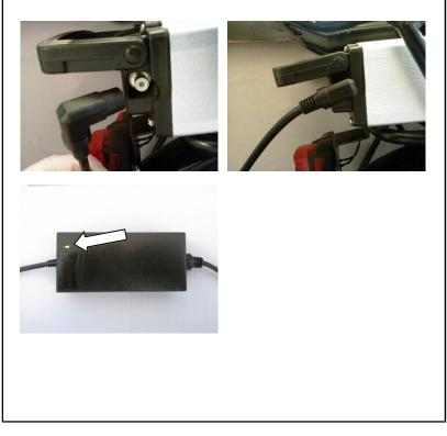
To remove the battery from your electric bike, use the supplied key to first turn **off** the battery by turning it anticlockwise to the "OFF" position, and then unlock the battery by pushing the key inwards and then turning it anti-clockwise again. Once unlocked, **remove the key** and then slide the battery from the bike using the handle as shown.
