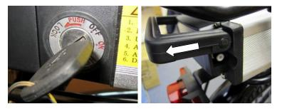
To refit the battery, simply slide it back into place, and then insert the key and turn it clock-wise to the "OFF" position to lock the battery in place, or if you want to use the bike immediately, turn it fully clock-wise to the "ON" position.
