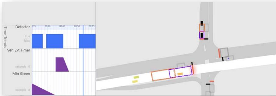
**Figure 26: Actual detector locations and TrafficSense detector locations.**
