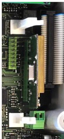
The receiver can also be retrofitted or replaced. This receiver can also be combined with an external antenna to be connected to the plug-in terminal directly under the module.
