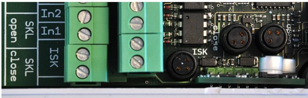
Illustration 8: Electrical connection of anti-crushing safety protection devices and ISK
