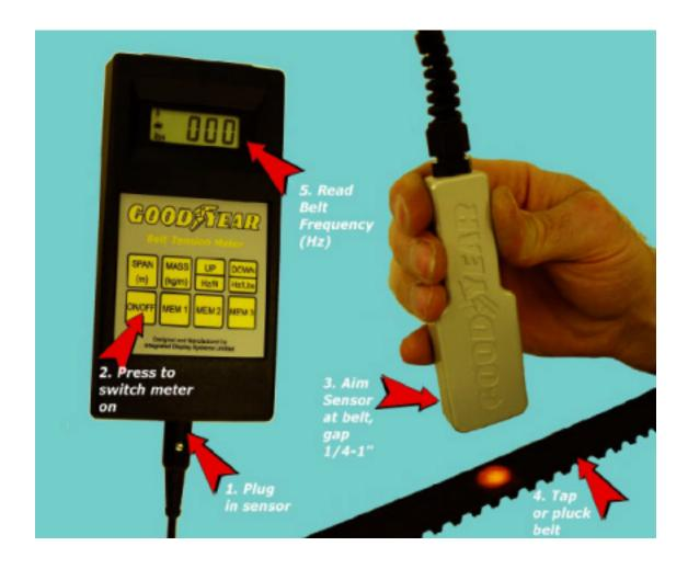
Following these simple steps will allow you to measure the vibration frequency of the belt. This value is independent of span or mass values but is very useful as an index for belt system maintenance, sometimes the only number you will need. For example, the MAXIMIZER $^{\text{m}}$  drive analysis program gives tensioning targets in Hz as well as in force units (newtons and pounds-force).
