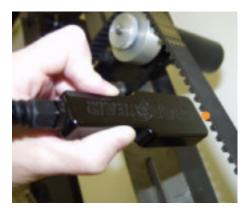
It is possible to take measurements from the edge of the belt. The toothed side of a belt is equally acceptable as a target for the sensor.
