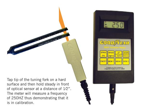
Results within  $\pm$  1% are acceptable. There is no adjustment possible. If greater variance is experienced, meter should be returned for recalibration. See Section 8.2 for recalibration return procedures.
