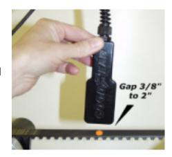
When physical restrictions are present, it is possible to get useable readings with the sensor at up to 2" distance from the belt and/or tipped up to 45 degrees from perpendicular.
