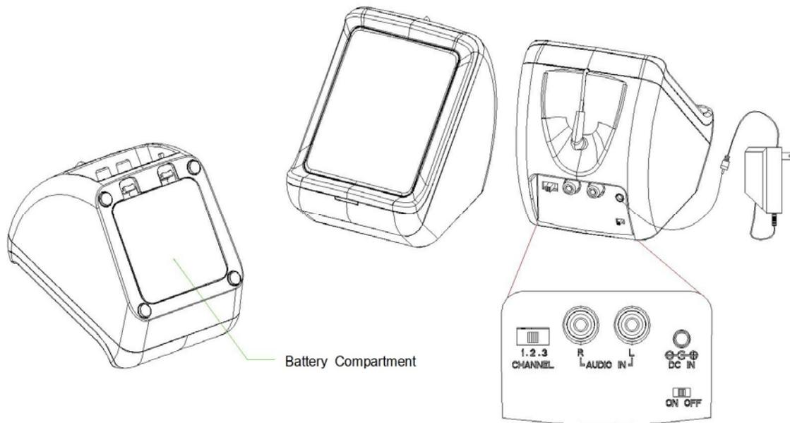
Turn the switch to On and the LED of the transmitter will light up in Green. When the audio cable has been connected turn on the audio source to at least a midrange volume level and play the music. The LED will turn from Green to Blue (Note: if the audio source is not in the play mode the LED will not turn from green to blue). If a speaker is not turned on within 4 minutes the transmitter light will turn from Blue back to green to save power.
