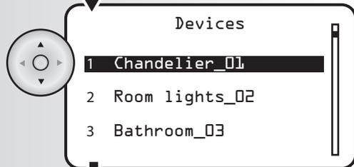
4. Using the arrow pad, highlight the desired destination device. A checkmark indicates associated devices. Press the OK button to Associate or Disassociate devices. To save the association, press the Menu button. To create additional associations, repeat steps 1-4.
