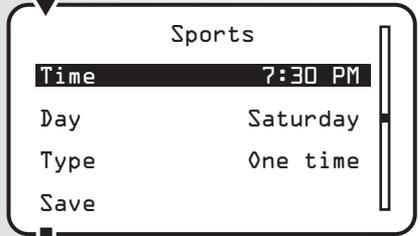
• Once you are in the time settings, the hour number will be flashing slowly. Use the up or down arrows to select the correct hour, then use the right arrow to proceed to the next hour, then to minutes, then select AM or PM. Press the OK button to save. **Note:** To enter 8:30 AM the user must enter 08:30 AM
