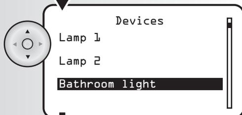
4. Use the left arrow to scroll left and erase the existing name (or portion of it) and then scroll up/down to enter the new name. Press OK to save the new name.
