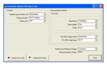
The controller system setting screen can be displayed from the "Controller system setting" of the system menu on the main screen.
