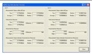
The below values for OUT1 and OUT2 are displayed at this screen. Maximum value, minimum value, average value, and medium value are calculated from the buffering data.
