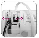
Plug the power supply C into the Alere Cholestech LDX® Analyzer and the wall or power strip. Insert the end of the white printer cable **D**. labeled 'To Cholestech LDX®," into the analyzer. Loop through the cable support.
