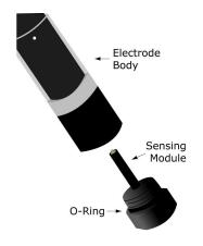
Install the replacement sensing module into the electrode body by screwing the sensing module until it is hand tight.
