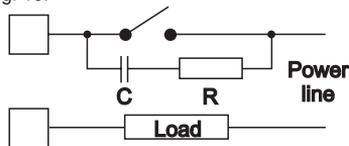
Fig. 10 EXTERNAL SWITCH IN SERIES WITH THE INTERNAL CONTACT
