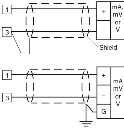
Fig. 6 mA, mV AND V INPUTS WIRING
