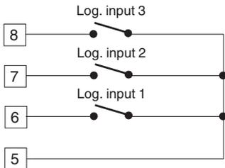
Fig. 7 - LOGIC INPUT WIRING
