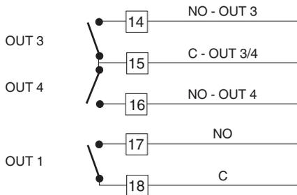
Fig. 9 RELAY OUTPUTS WIRING
