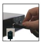
Connect the cable of the power supply to the Freecom DVD RW Recorder and the power supply itself to the socket.
