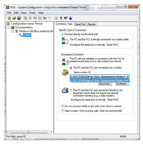
Select the modem you want to use for the connection (in this case GVC 33.6K External..... Modem) and continue to set up modem specific parameters by pressing the "Configure..." button. The options available in the "Configure" popup dialog differs among modem vendors but typically baud rate, flow control, additional AT modem commands, compression and other hardware parameters can be set up using the "Configure..." dialog.
