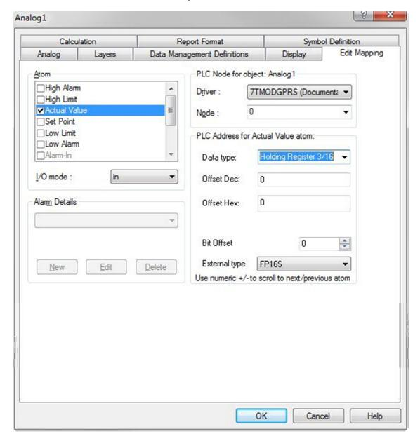
Now select the desired PLC node number and continue by setting be desired Device. Then specify the number (register number within the device type). Note that the corresponding Mnemonic is displayed and updated as you select the appropriate parameters. This is a help to make sure you always bind to the correct process variable.
