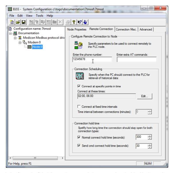
In the "Connection Scheduling" section you can design a connection schedule either by entering specific points in time during the day where the driver will establish connection or you can enter a fixed time interval where the driver will establish connection – or a combination of both specific points in time and fixed intervals.
