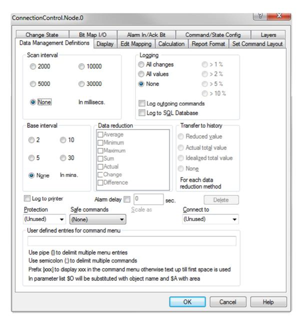
And bind both the Command- and the State atom to "Historical Data (Word)" and Word Offset 0 (this corresponds to parameters 0 and 0 we just set up in the "Connection Misc." pane for the driver).
