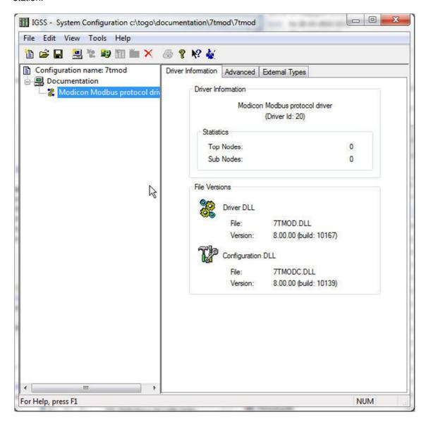
When the driver has been added to the relevant station you are ready to add and set up the interface and PLC nodes.
