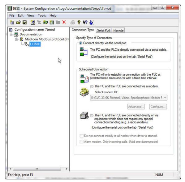
The Modicon Modbus Serial driver is designed to use either direct serial communications or modem/radio and thus you should select one of the options:
