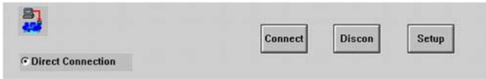
The direct connection area of the screen allows you to link directly to the CCS master using an RS-422 interface board in the PC. The direct connection command buttons are as follows:
