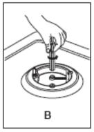
o Unscrew the injector **(B)** and replace it with the stipulated injector for the new gas supply (see the table on the next page).
