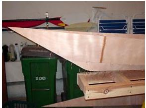
The side panels wired to the bottom panels at the bow.
