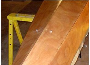
The screws used to hold station #5 until after the first layer of fiberglass hardens on the outside of the hull. Note that in this photo the first layer of fiberglass is on the hull, which is a later step.
