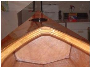
The filled gap in the front of the coaming.
