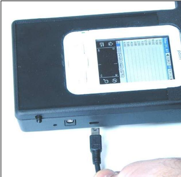
Connect the Mini USB connector to the IDvisor.
