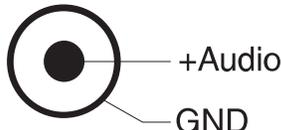
Figure 9. GT724 auxiliary equipment RCA jack
