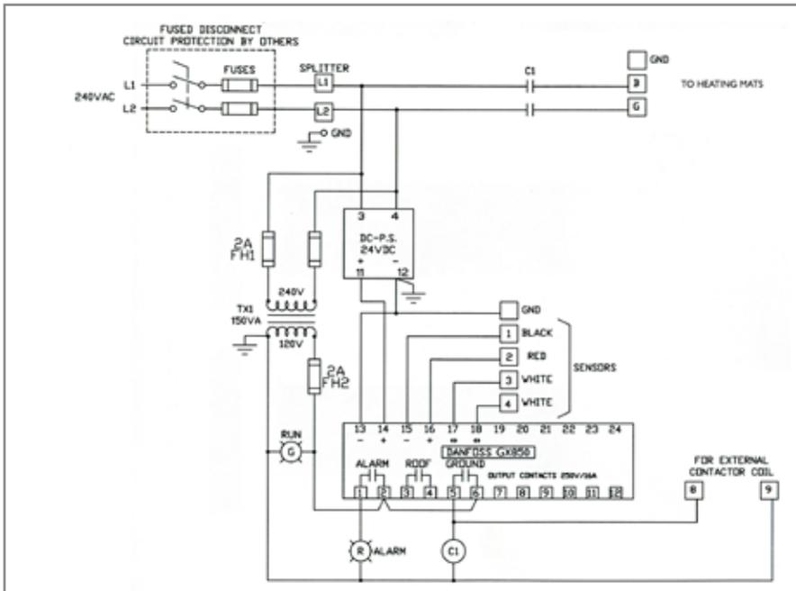
The GX™ 850 has an integral alarm function that monitors the attached sensors and the in-built microprocessor.
