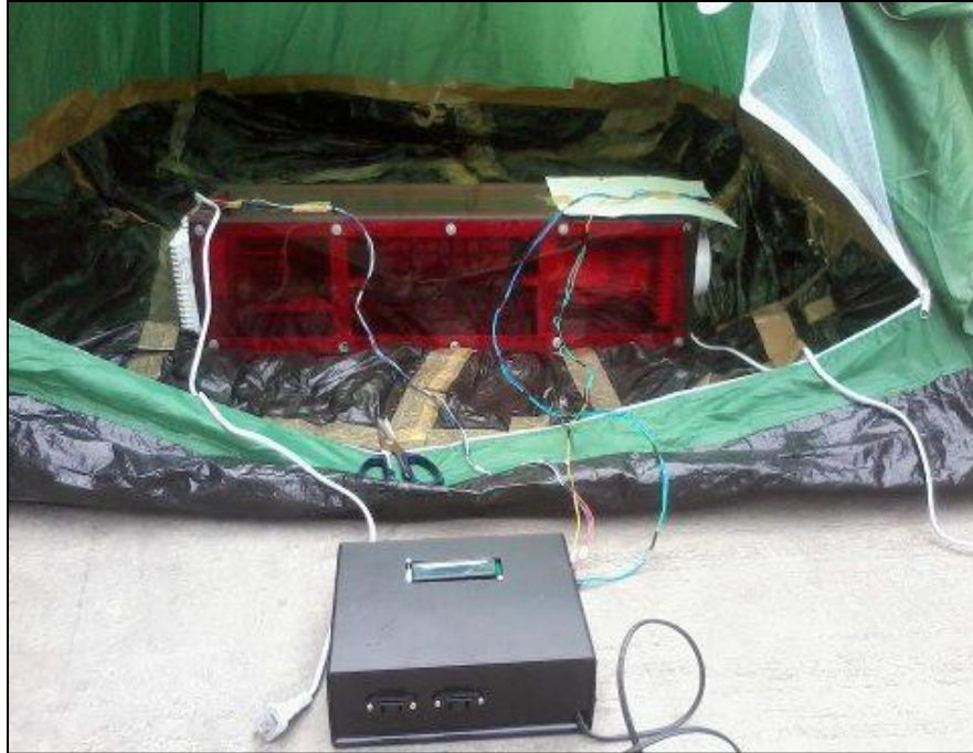
Picture 3: Complete Setup of Carbon Monoxide Converter with Catalytic Converter
