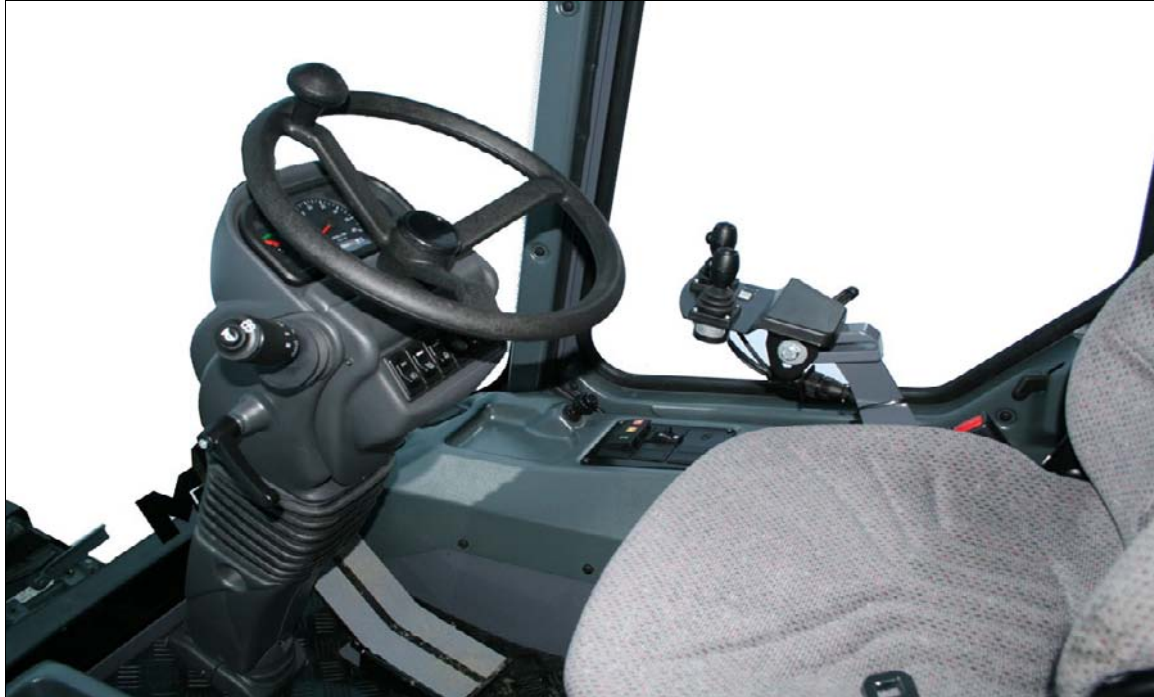
STEERING COLUMN, RIGHT SIDE PANEL, HAND GAS AND RIGHT ARM SUPPORT
