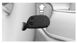
The lever automatically returns to its initial position when released.
