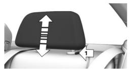
The height of the outer head restraints can be adjusted.
