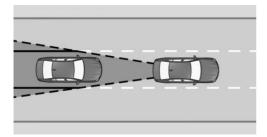
Two radar sensors in the rear bumper monitor the area behind the vehicle.
