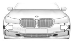
With the respective equipment variant, there are two additional radar sensors in the front bumper.
