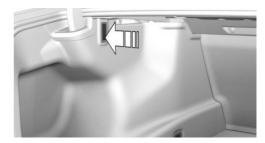
A multi-function hook is located on the left side in the trunk. Press on the multi-function hook and turn until it engages.
