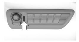
Thumbwheel for changing the air flow direction.
