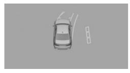
Obstacle markings are displayed sideways on the vehicle to protect the vehicle sides.
