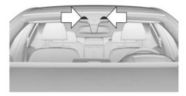
The camera is installed near the interior rearview mirror.
