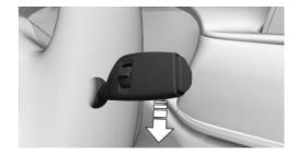
After the wipers are folded back down, the wiper system must be reactivated.
