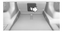
Pull on the rear handle and push the cooler into the guide rails.
