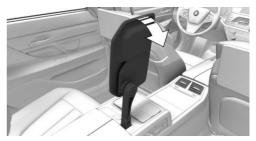
The folding table can be rotated by 90° or 180° to the left and can be enlarged.
