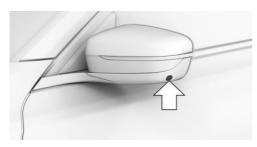
There are two cameras at the bottom in the exterior mirror housings.
