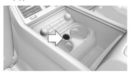
The socket is located between the cup holders under the cover.
