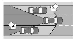
Two radar sensors in the rear bumper monitor the area behind and next to the vehicle starting from a preset minimum speed.
