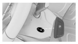
If a respective Check Control message appears, hold the remote control with its back against the marked area on the steering column. The tailgate button on the remote control should be at the same height as the marked area. Press the Start/Stop button within 10 seconds while pressing the brake pedal.
