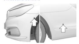
With the four side ultrasound sensors, arrows, and the ultrasound sensors of the PDC in the bumpers, the parking spaces are measured and the distances to obstacles determined.
