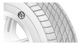
RSC label on the tire sidewall.
