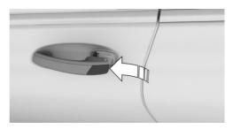
Guide one finger of the other hand from the back under the lid, push the palpable release outward and remove the lid.
