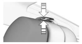
The head restraint folds into the topmost position. Close the pushbutton on the lower tab and the pushbutton on the bottom of the head restraint.
