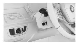
The light switch elements is located next to the steering wheel.
