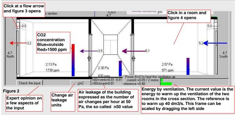
The 6 arrows indicate the ventilation flow rates in the cross section of the building. The size of the arrows is the relative size of the flow. During the CO<sub>2</sub> simulation the arrows are colored from blue =
