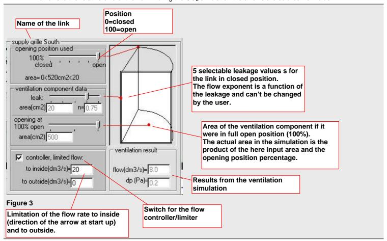
outside concentration to red=1500 ppm. A click at an arrow yields the input frame of figure 3. The mouse can drag these frames. The top edge border is the best place to drag the frame. You can't drag the frame by clicking on the internal elements(sliders, internal frames and textboxes)
