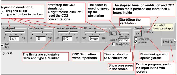
Here are controls for: wind speed, wind direction, temperature and outside CO<sub>2</sub> concentration
