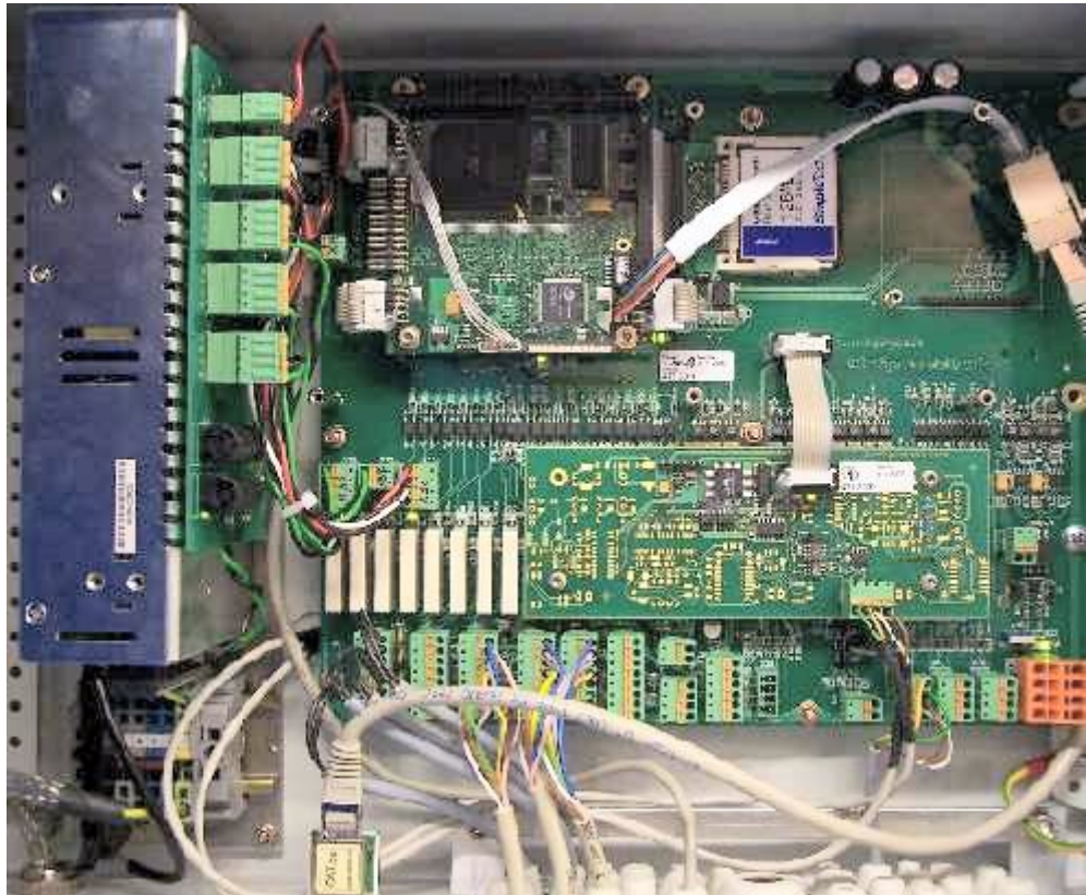
Fig. 3.2: Internal view of the control section (single-stream system) without cover
