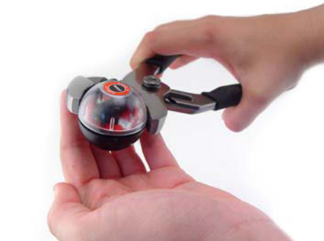
2. Apply light pressure at equator of sonde with pliers to disengage snap.
