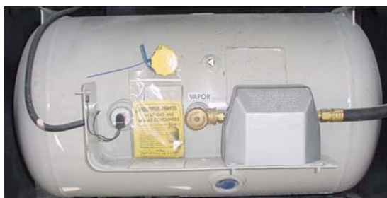
Figure 3-6. Liquid Propane Tank
