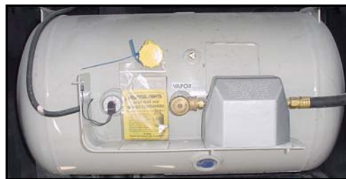
Figure 2-4. Liquid Propane Tank
