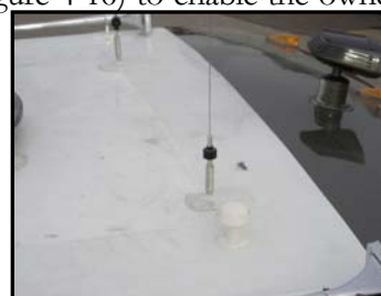
Figure 4-16. CB Antenna Installation
