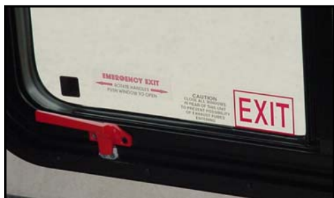
Figure 13-2. Emergency Exit Window
