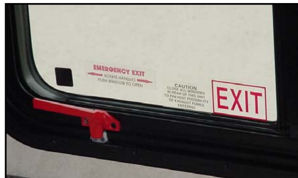
Figure 2-9. Emergency Exit Window
