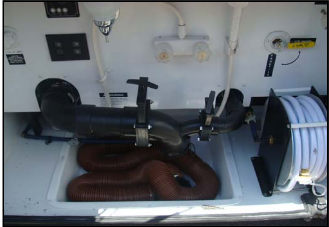
Figure 11-12. Sanitation Compartment Containing Holding Tank Drains and Flexible Drain Hose
