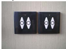
Figure 10-6. Control for Passenger & Entry Door Power Shades
