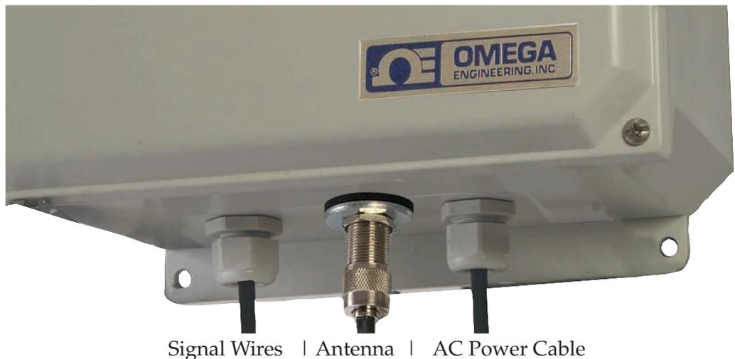
**Figure 4-1. HPWS Enclosure Connections**
