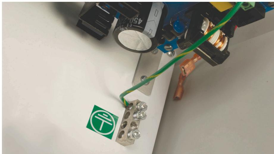
Figure 3-5. Grounding Bus Bar Connection
