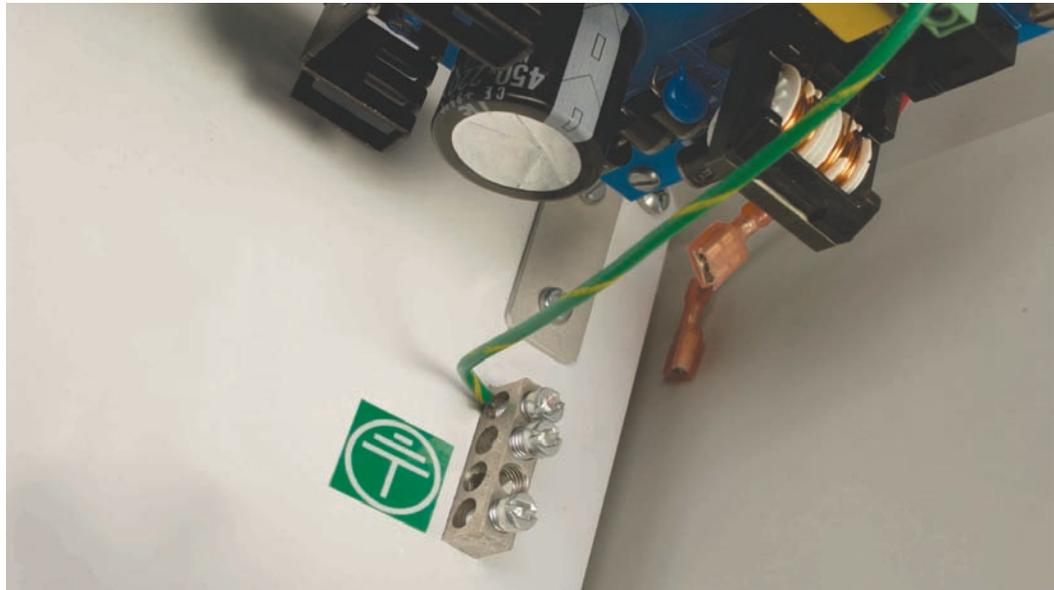
**Figure 4-3. Grounding Bus Bar Connection (Model HPWS-REC)**
