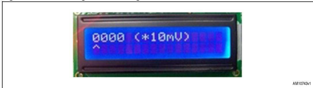
The UP and DOWN switch sets the number. To move to the next digit, press enter.
