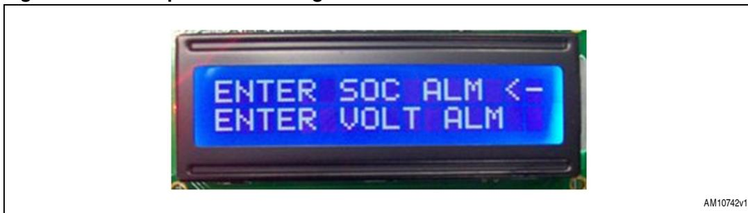
To enter the battery LOW SOC Alarm, select the "Settings" tab and select the appropriate option. Now the user is able to see the image shown in [Figure 15](#).
