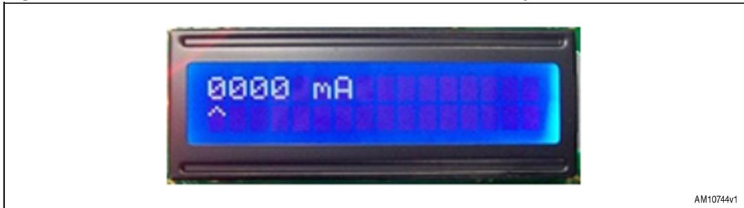
Using the UP and DOWN switch sets the number. We can enter this threshold value in multiples of 20 mA only. To move to the next digit, press enter.
