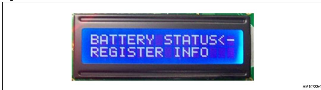
While scrolling through the menu, (by pressing the menu button or navigation buttons) one of the options is always indicated by the arrow mark "<-", as shown in [Figure 9](#). By pressing the enter key the corresponding tab is selected, which is indicated by the arrow mark "<-".
