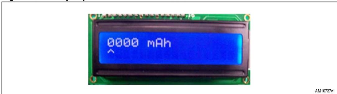
Using the UP and DOWN switch sets the number. To move to the next digit, press enter. When all the digits are set the user is able to see the image shown in [Figure 16](#):
