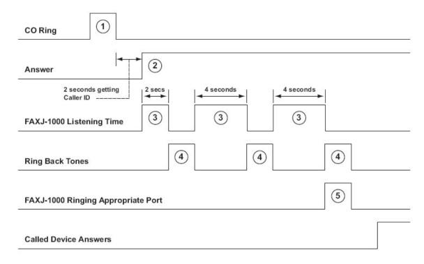
**Note:** If fast call processing is enabled (see Programming section C), the second 4-second listening time is eliminated, so that the FAXJACK rings the appropriate port after the first 4-second listening time. Enabling fast call processing can make it more likely for a fax call to be incorrectly routed to the Phone 1 port because CNG tone is not detected.
