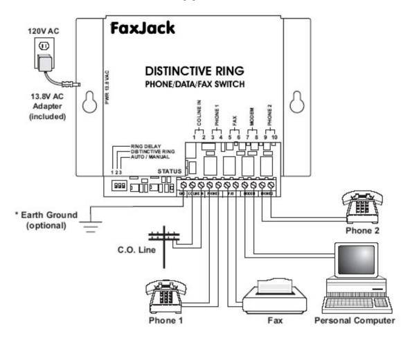
Note: The polarity of the connection to the CO Line In terminals shown to the right should be (+) or Tip to terminal 1 and (-) or Ring to terminal 2. Observing this polarity helps prevent clicks and dings of connected phones on hang up.
