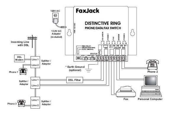
The **FAXJACK** is designed to be wired at the Demarcation Point (the point where the phone line comes into the house), but in some cases this may not be possible or convenient. This section shows a way of hooking up the **FAXJ- 1000** to any existing phone jack, provided the house is wired for at least two lines. A splitter/adapter is required for each jack in the house (ie: Radio Shack part # 279-402).
