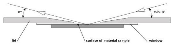
At very positive potentials, the Beryllium window may suffer from oxidation. In this case we recommend placing a thin insulation layer, e.g. a small piece of polyethylene foil (15 mm in diameter, 10  $\mu$ m thick), in between the holed current collector and the Beryllium window.
