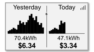
The graphs show hourly data, with a bar for each hour. The height of the bars is proportional to the number of kWh consumed for each hour. The graphs are autoscaling, and meant to show relative, rather than absolute values. The small number near the top of the center line indicates the value (in kWh) of the highest bar in the graphs.
