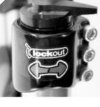
If you have an O<sub>2</sub>4u with lockout you can lock the fork by turning the lockout dial 90 degrees counter clockwise. Turn it back again to unlock.
