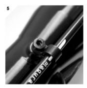
To use the disc tube guide, first clamp the tube in the guide as shown
