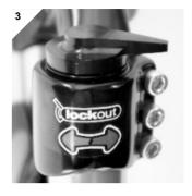
**3** If you have a 2-Stroke with lockout you can lock the fork by turning the lockout dial 90 degrees counter clockwise. Turn it back again to unlock.
