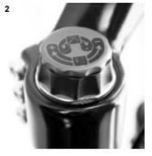
On the right leg another dial is placed on top of the preload dial. This dial is to adjust rebound damping. Turn the preload dials clockwise to add preload. Turn them counter clockwise to remove preload. To increase rebound damping, turn the rebound-dial clockwise. To decrease rebound damping, turn the dial counter clockwise.
