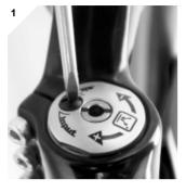
To adjust the air pressure, first remove the cap of the air valve with a small screwdriver.
