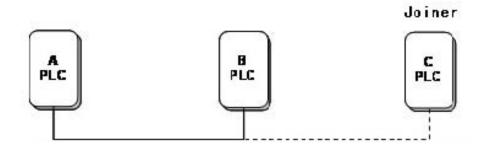
Do as follows to add device C to network N using the Security button:
