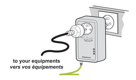
Recommended use of a multiple plug adapter, Place the PLC taken first on the multiple plug adapter.
