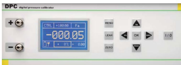
Press the MENU button and then press the UP / DOWN until you are on the desired sub menu. With OK you go into the appropriate sub menu. The following items in the submenu are available:
