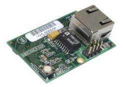
There is one difference between the mapping of the Disk-on-Module device and that of the QEM: while the IDE device is mapped into CS5 memory space, QEM is mapped into CS4 memory space (it is addressed by the address signal lines A1 and A21), but both devices use the same interrupt signal. Address line A21 selects whether the DoM Ethernet chip or secondary Ethernet (connected via SO-DIMM bus interface, e.g. QUANTUM Base Board V2) is selected (by CPLD).
