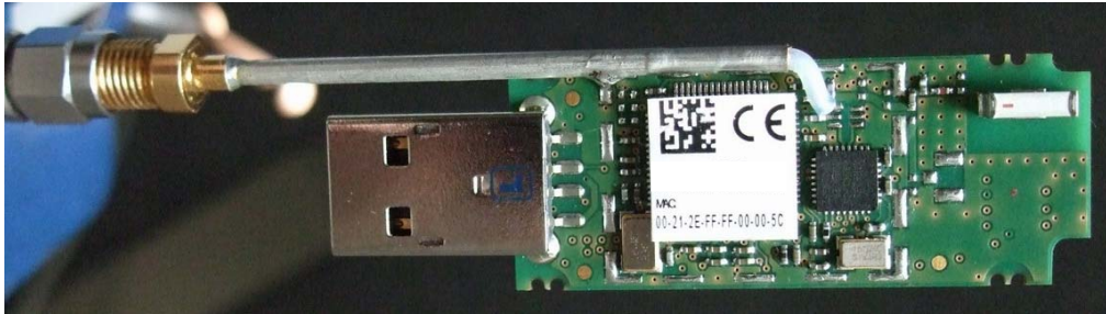
Figure 5-9. Antenna tuning test board (without RF shielding).
