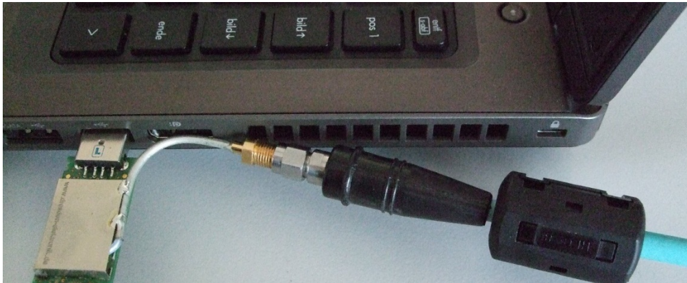
Figure 5-10. DUT with metal shielding plugged into laptop, coaxial cable with ferrite bead.
