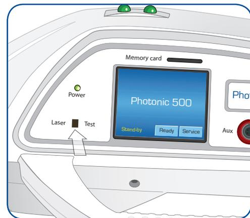
„Laser Test“ sensor on the front panel
