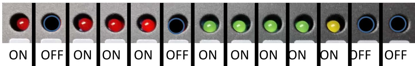
In the case the unit displays very dim images, the LED readout above indicates there is most likely an issue in the backlight lamp.
