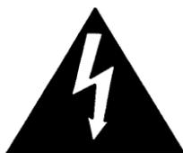
This symbol is intended to alert the user to the presence of insulated “dangerous voltage” within the product’s enclosure that may be of sufficient magnitude to constitute a risk of electric shock to persons.
