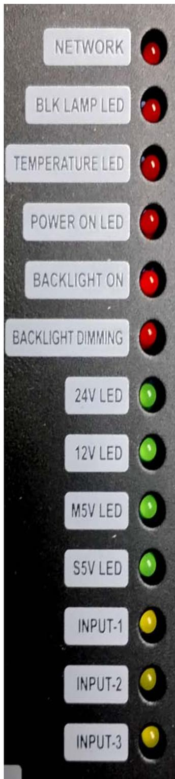
Network (red): indicates whether the ACR has LAN connection. The light will be on if the SMC is connected to a network device. This does not necessarily indicate internet connectivity.
