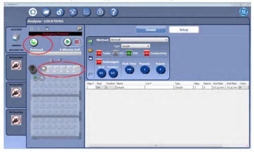
• Load the sample vials into the Emergency Protocols rack located in front of the GE Autosampler tower. Click the corresponding positions on the Emergency Rack graphic and apply the appropriate method to each vial.
