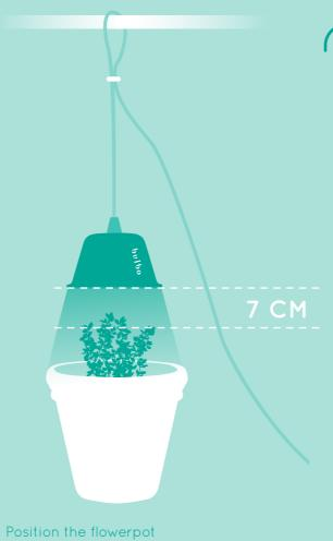
directly under the illuminating beam of the Cynara.
