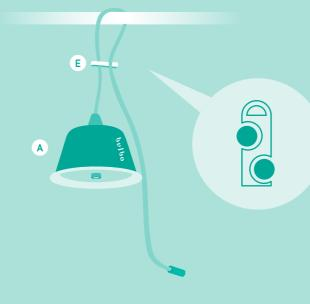
Create a loop with the power cable of the device, letting it pass around the support on which you would like to hang the Cynara.
