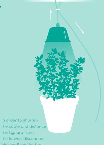
the cable and distance the Cynara from the leaves, disconnect blocker **E** and let the cable slide downwards.
